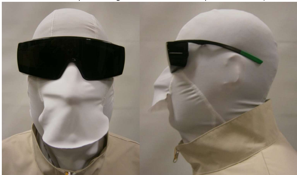
Fig.6 UV-protection glasses at the UV-head protection mask front- and side- view
